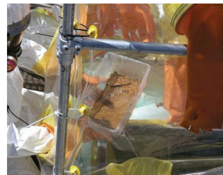
A sample of rust-colored sludge dredged from one of the tanks. The scaffolding in the foreground supports a portable glovebox-like sampling apparatus designed to protect the researchers and samples from contamination.
