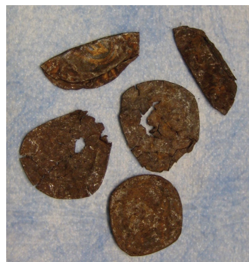
Rusty bottle caps collected from a parking lot at the former site of the Manhattan Project's D Building were analyzed for trace Pu contamination. The samples were found to contain ^{240}\text{Pu} - ^{239}\text{Pu} isotopic ratios characteristic of Pu from the earliest years of the U.S. nuclear weapons program.
