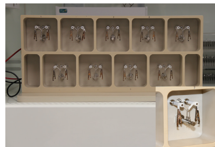
TIMS filament-electroplating system. The inset shows a close-up of a filament set up for sample electroplating.
