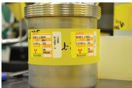
Examples of the various sample geometries encountered during NDA by gamma-ray spectroscopy.
